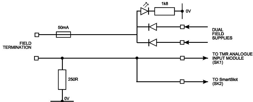
The T8831 is similar but replaces the fuse with a resistor, limiting available power for non-incendive applications (non-incendive hazardous area specifications specify limited loop power and are used in the Americas).
