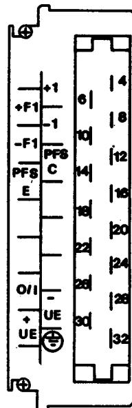
The module supplies automation systems with 5 V DC from a main supply of 24 V DC. It is a DC/DC converter with safe isolation between input and output voltage. The module is equipped with overvoltage protection and current limitation. The output is short circuit proof.
