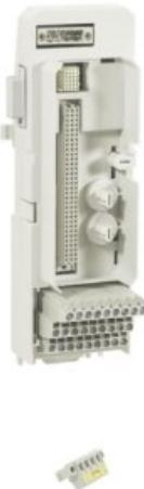
The TU891 MTU has gray terminals for field signals and process voltage connections. The maximum rated voltage is 50 V and maximum rated current is 2 A per channel, but these are primarily constrained to specific values by the design of the I/O modules for their certified application. The MTU distributes the ModuleBus to the I/O module and to the next MTU. It also generates the correct address to the I/O module by shifting the outgoing position signals to the next MTU.
