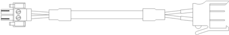
Figure 516 Layout of the FS-PDC-MB24-y power distribution cable
