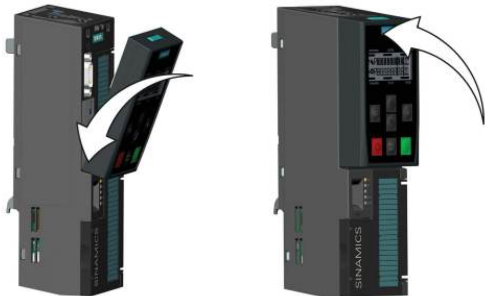
Image 5-1 Fitting the BOP-2 to the Control Unit
