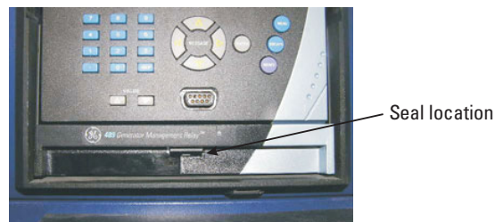
FIGURE 3-2: Drawout Unit Seal
