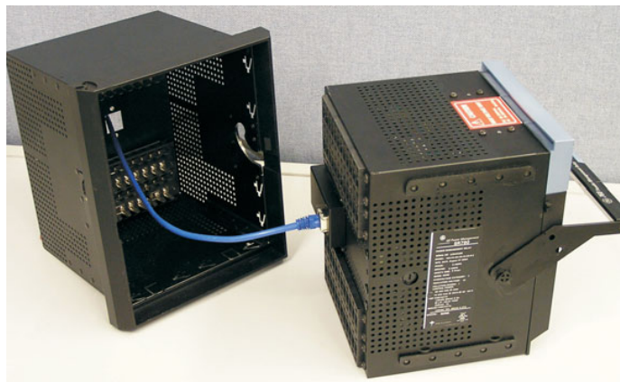
FIGURE 3-8: Ethernet Cable Connection
