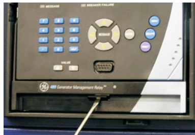
FIGURE 3-5: Press Latch to Disengage Handle
