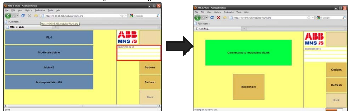
Figure 25 MView Redirecting to Redundant MNS Digital Gateway
