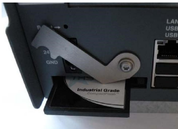
Figure 8 CF Card Insertion Detail
