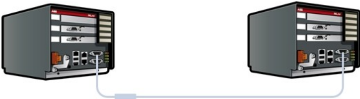
Figure 22 Serial 1 to serial 1 redundant link connections with ferrite core
