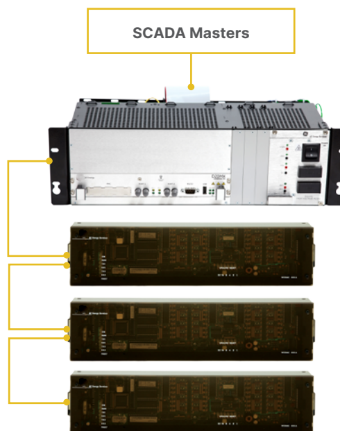
Figure 1: Simple architecture of I/O modules communicating to the D20 RTU
